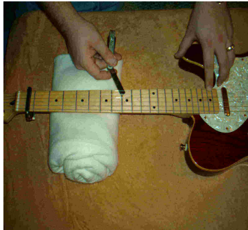
Use Feeler Gauge to measure the gap between the string and eighth fret while fretting the string at last fret. Gap should be approximately .010".
