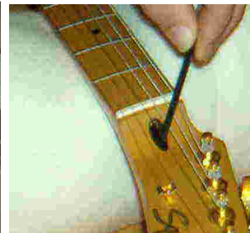
Adjust Truss Rod accordingly
