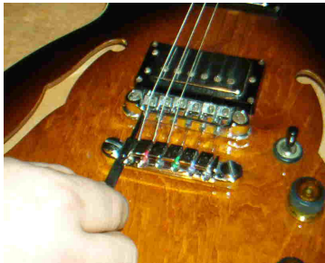
Left picture: Tuneomatic style bridge. Use a small flat head screwdriver to make saddle adjustment.
